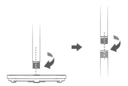
2. Insert the fan head pole into the upper pole (2) and turn clockwise until tight.
