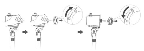
4. Install the rear grille (5) onto the fan head as shown below. Replace the grille nut (6) and turn clockwise to secure.
