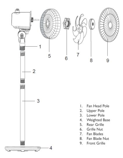
1. To set up the fan as a pedestal fan, insert the lower pole (3) into the base (4) and turn clockwise until tight. Then insert the upper pole (2) into the lower pole (3) and turn clockwise until tight.
