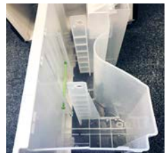
You can now access inside of water tank
